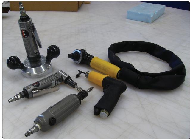
Figure 7-32. Air tools used for composite repair.
