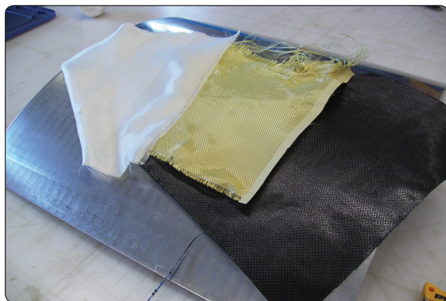
Figure 7-7. Fiberglass (left), Kevlar® (middle), and carbon fiber material (right).
