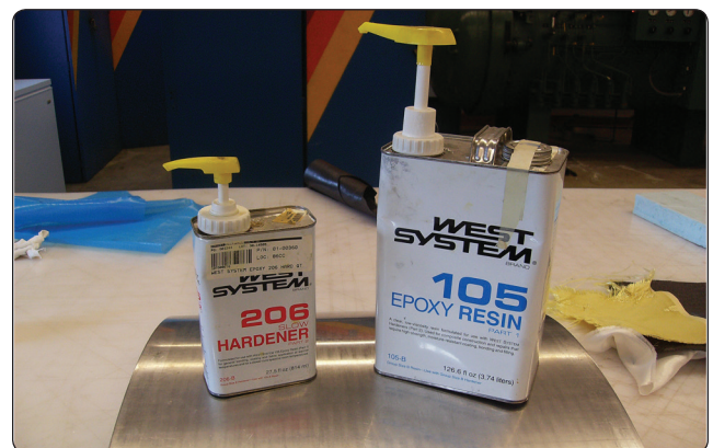
Figure 7-10. Two-part wet layup epoxy resin system with pump dispenser.
