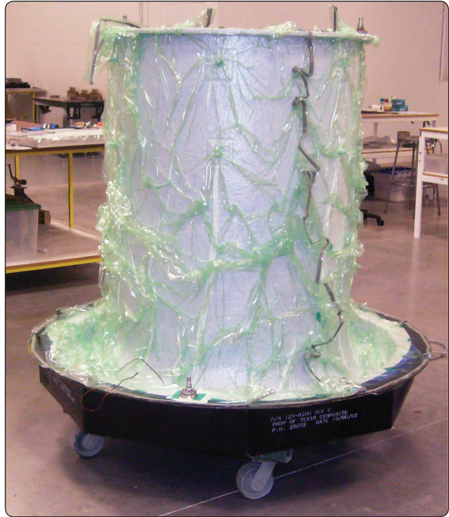
Figure 7-36. Bagging of complex part.
