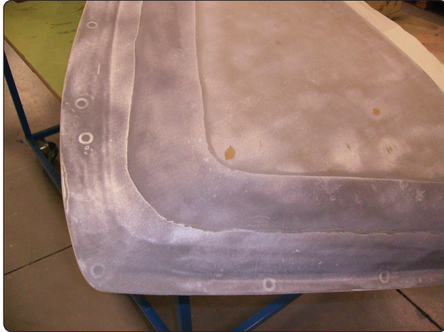
Figure 7-9. Aluminum mesh lightning protection material.
