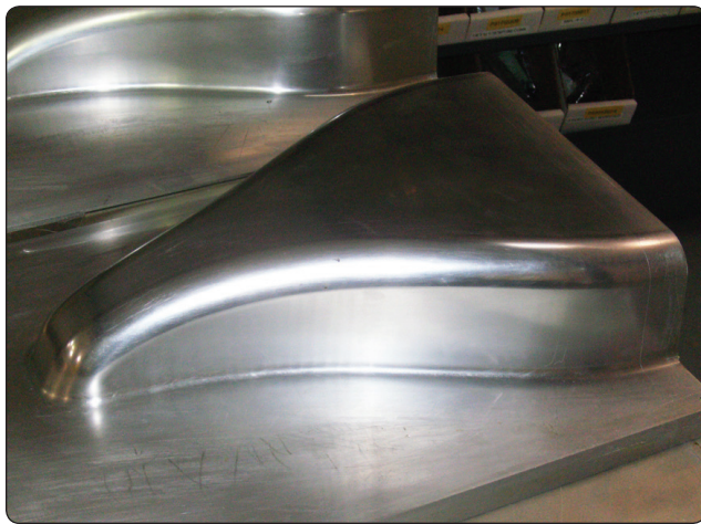
Figure 7-34. A mold of an inlet duct.
