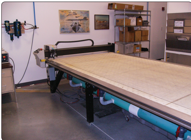
Figure 7-89. Gerber cutting table.
