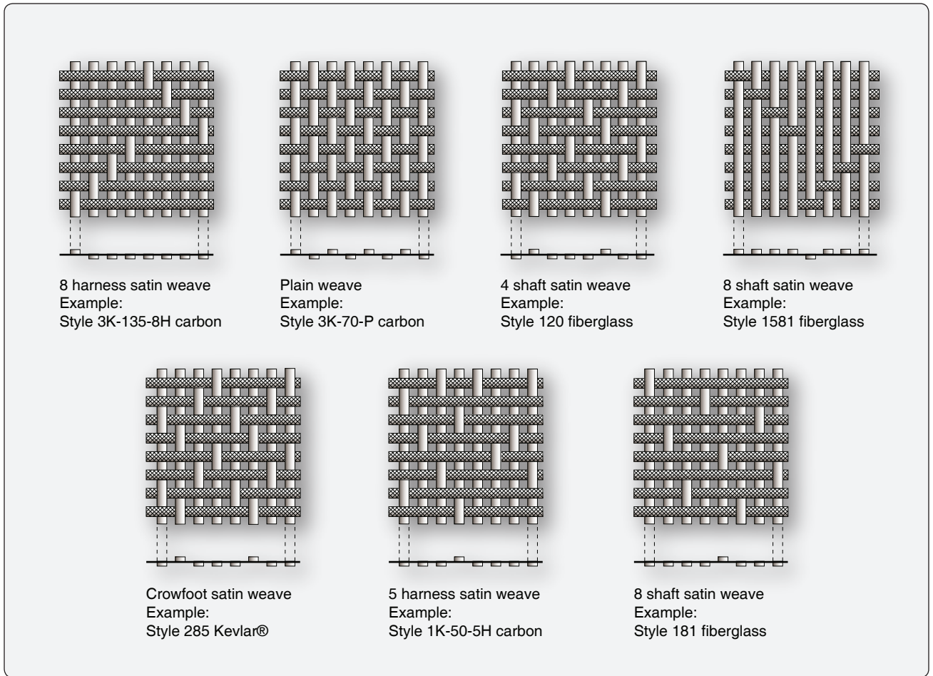
Figure 7-5. Typical fabric weave styles.
