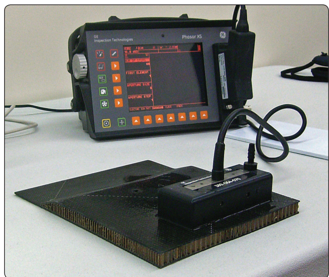
Figure 7-28. Phased array testing equipment.
