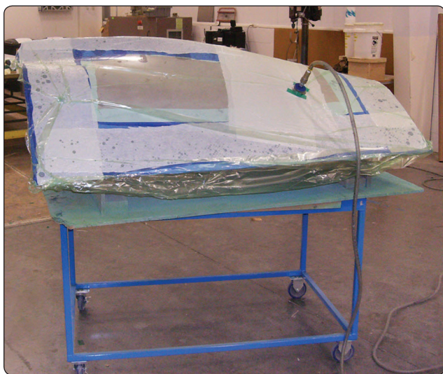
Figure 7-52. Envelope bagging of repair.
