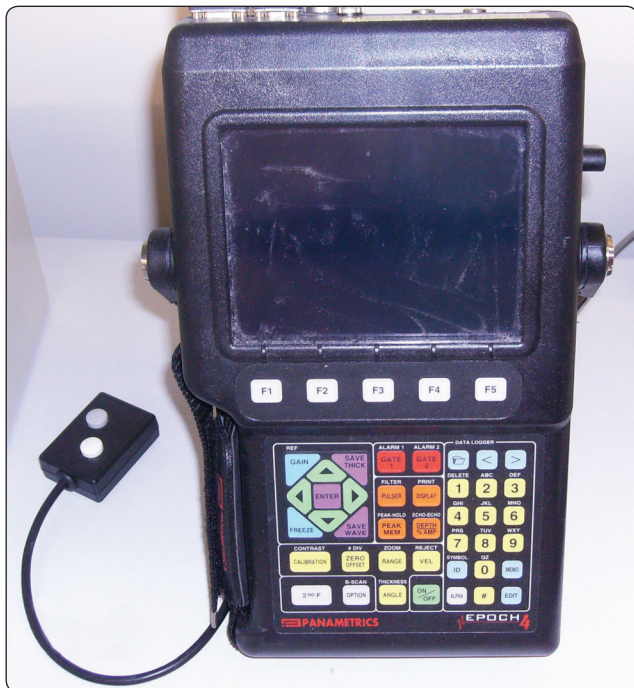
Figure 7-26. Pulse echo test equipment.
